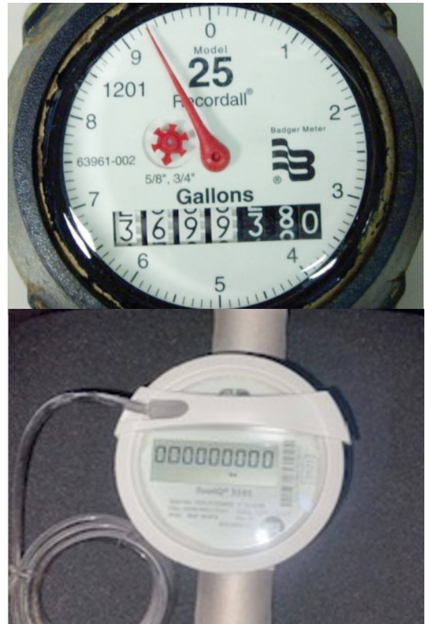
Figure 1-12: Straight-reading meters in gallons (upper) and cubic feet (lower)
